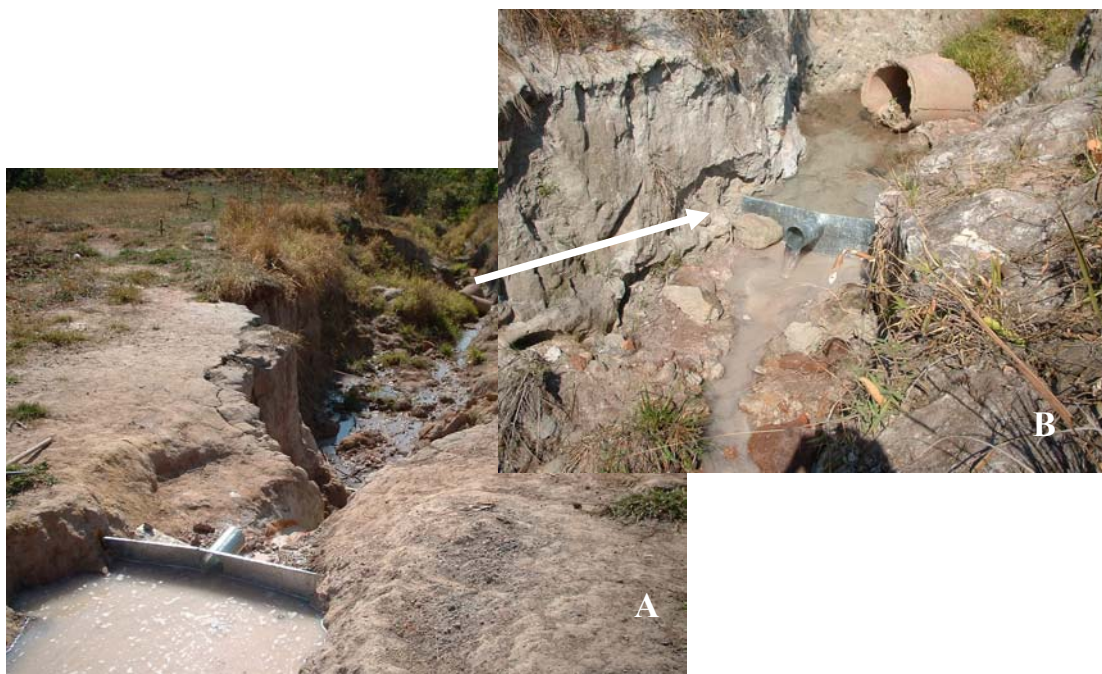
Fig. 2 – This picture shows the two points of water flow variation data collect. The figure A indicates where was the point 1, which was located before the water fall. The figure B indicates where was the point 2, which was located near of the gully mouth and is indicated by the white arrow. It was used about 25 minutes in each point for installing and starting the process of data collection (ALVES, Ricardo – October 2003).
