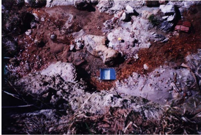
Fig. 3 – Sediment trap installed at the bottom of the gully's channel (ALVES, Ricardo – September 2003)
