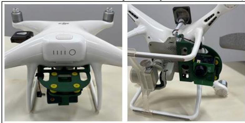
Figure 2 - Phantom 4 PRO with Mapir Survey 3w camera mount (OCN)
