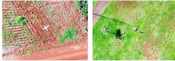
Figure 4 - Control point for georeferencing Ground control point Fixed point
