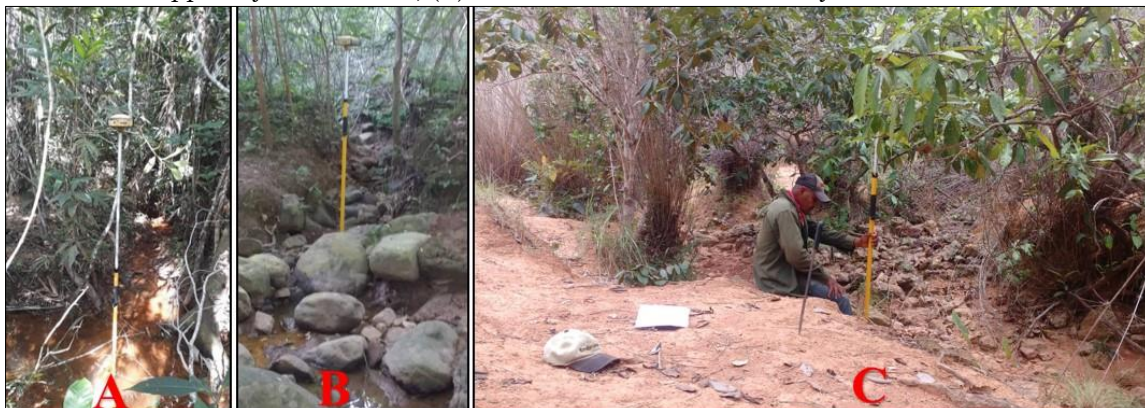
Figure 6 - (A) Coordinate collection in drainage mapped by ODR_Hidro; (B) Coordinate collection in bifurcation mapped by ODR-Hidro; (C) Coordinate collection at the junction of two bifurcations.
