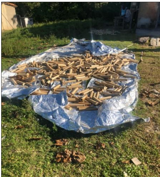
Figure 3 – Drying process of the taboca.
