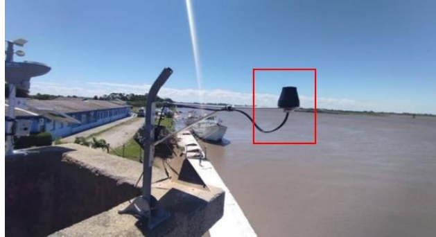
Figure 2 - Installation of the GNSS-R station in Rio Grande, highlighting the antenna (in red).
