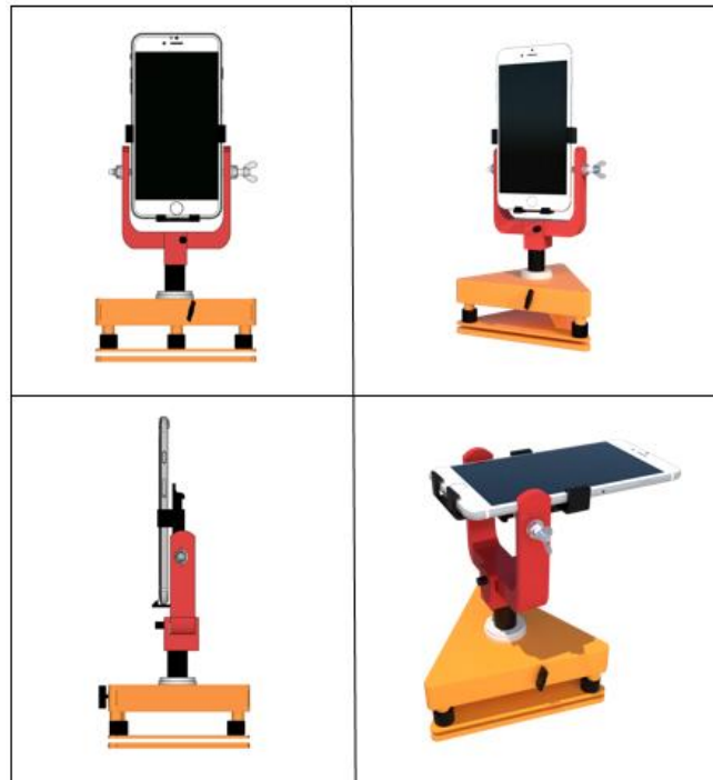
Figure 4 – Support developed for taking measurements with the smartphone attached to a base.
