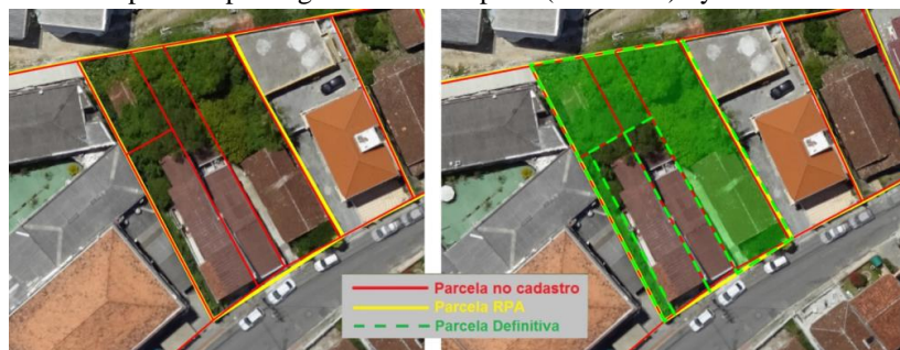
Figure 4 - Example of replacing non-certified plots (left in red) by a certified one. (right in green).
