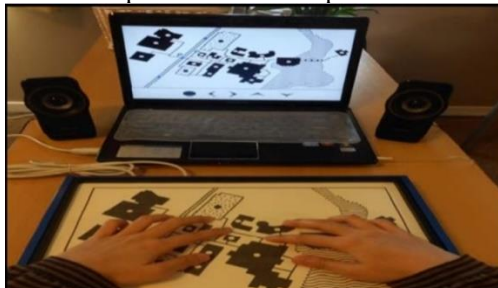
Figure 2 - Example of a Tactile map with sound features.
