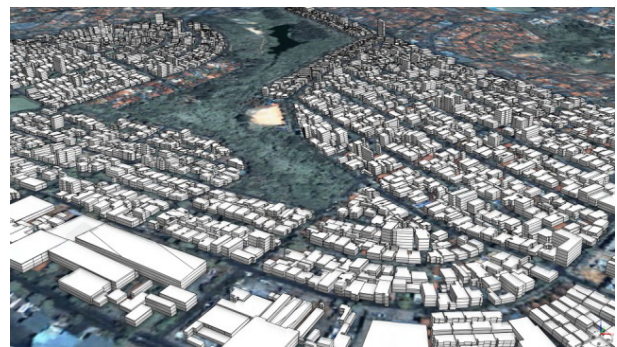
Fig. 15 – Simulation of volumes of existing buildings for the study area. Source: Elaborated by the authors, with data from Lidar dataset, 2016.
