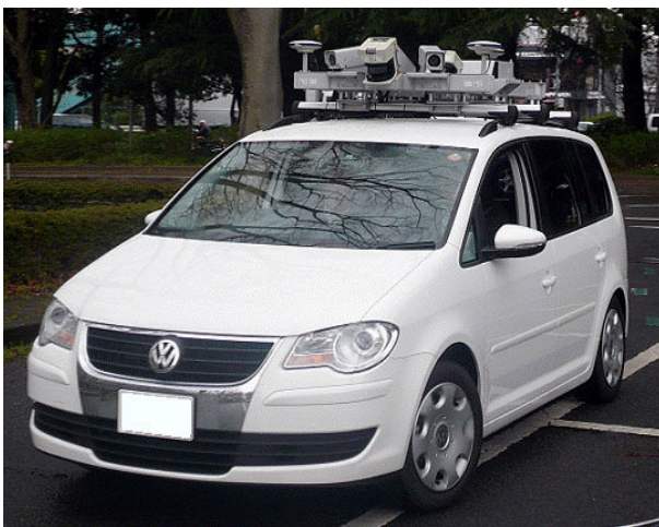
Fig. 4 - All direction MMS (PASCO, 2013).
