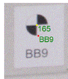
Fig. 14 - Projected surveyed target (red point) and its neighboring automatically-extracted target (yellow point).
