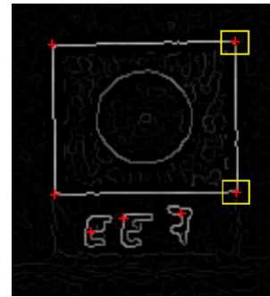
Fig. 5 - Accurate localization of identified corner points by the Förstner interest operator.
