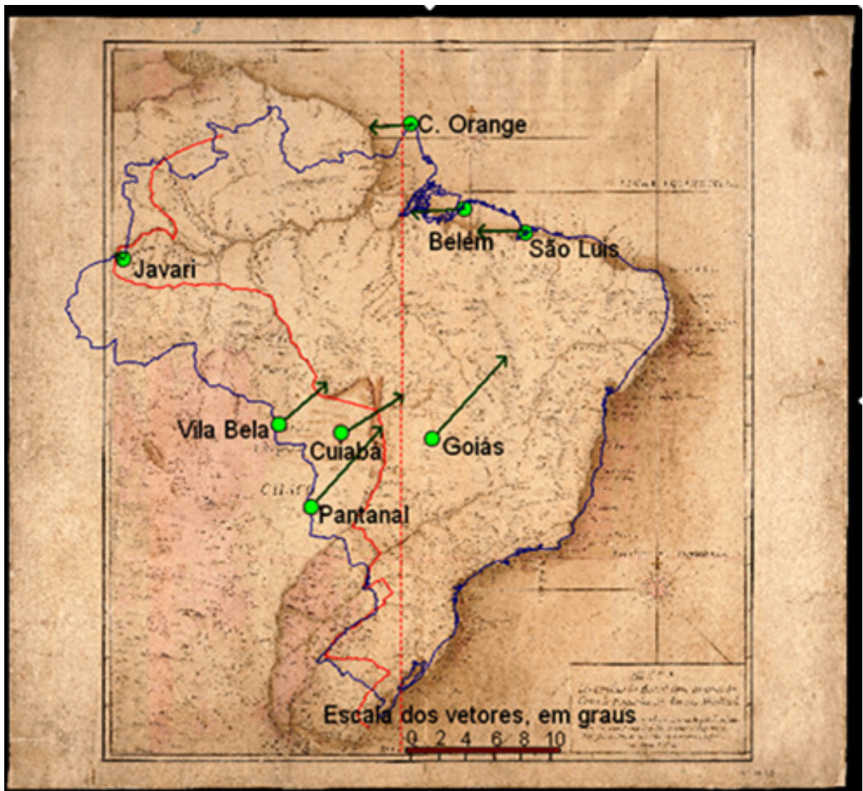
Fig. 20: Map of the Courts, with its distortions indicated by green arrows, distorted borders in red and real borders in blue.
