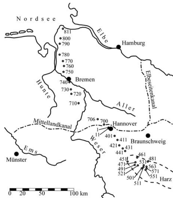
Fig. 3. - The station distribution of the gravimeter calibration system Hannover (Cuxhaven-Harz mountains, 3000 \mu\text{m/s}^2 , 90 \mu\text{m/s}^2 interval), e.g. TORGE, 1989.
