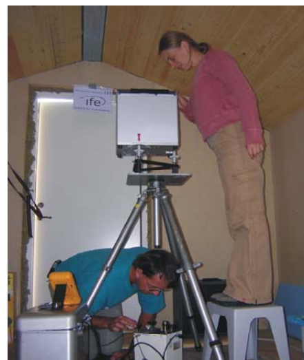
Fig. 7. - Simultaneous measurement of the vertical gravity gradient with LCR G709 with integrated SRW-feedback system, and with Scintrex CG-3M no. 4492. In a standard procedure, the difference is measured 10 times with each instrument.
