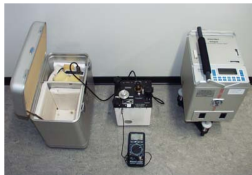
Fig. 1. - Scintrex Autograv CG-3M no. 4492 (right) and the LaCoste-Romberg model G no. 709 with carrying case (left).
