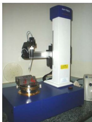
Figura 5: Circularímetro Talyrond 131 – Taylor Hobson
