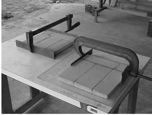
Figure 3 – Specimens for the guarded hot plate tests
