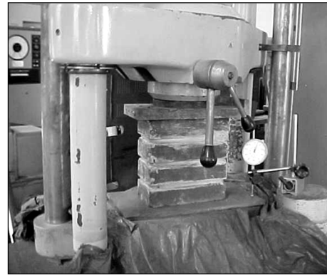
Figure 2 – Mini panels submitted to simple compression
