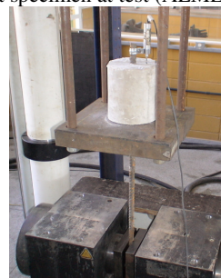
Figure 2 – Pullout specimen at test (ALMEIDA FILHO, 2006)
