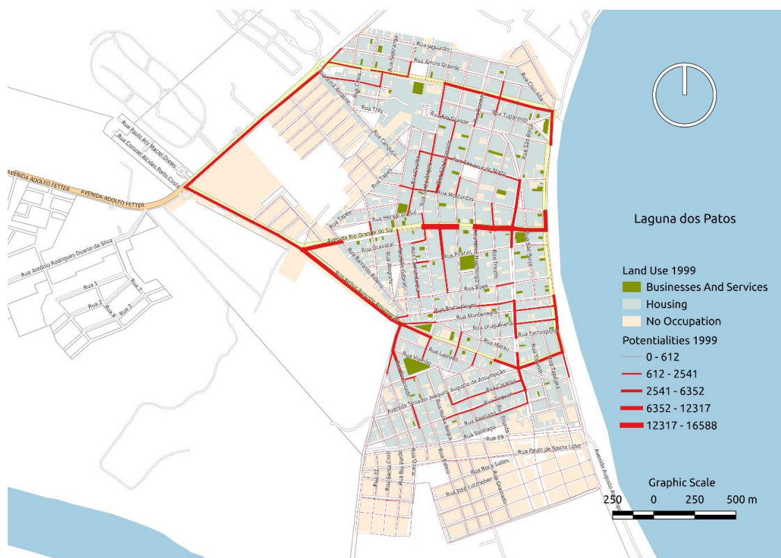
Figure 6 - Result of the Potentiality measure and land use for the year 1999, Laranjal/Pelotas, RS
