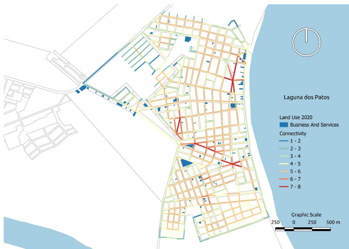
Figure 11 - Road system connectivity and location of businesses and services land uses for 2020, Laranjal/Pelotas, RS
