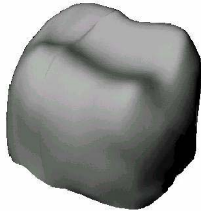
Figure 5 – Shaded NURBS surface fitted, curve-net based measurement with CMA.
